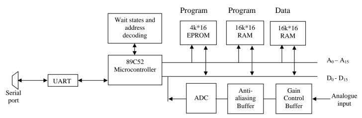
Figure 3 PC-based FFT spectrum analyzer hardware.
