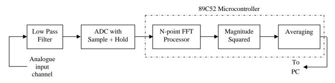
Figure1 the conceptual block diagram
