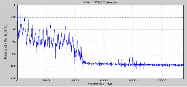
Figure 6 Frequency Spectrum of a woman speech signal. Minimum Power: -81.8281 dB, Maximum Power: 7.8951 dB, Average Power: -15.1359 dB, Signal-to-Noise Ratio: 63.6207 dB, Noise Floor: -54.0605 dB, Total Power: 10.8956 dB.
